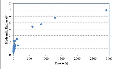
Figure 10-1. Velocity and Hydraulic Radius as a Function of Flow at USGS Gage 11105510
